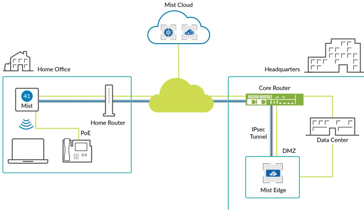
Figure 2: Extending the Enterprise with Mist Edge solution
